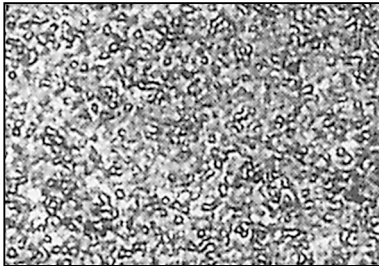
Finegrain-hardmetal structure Ultra-micro-grain, grain size 0–0.5 micron
